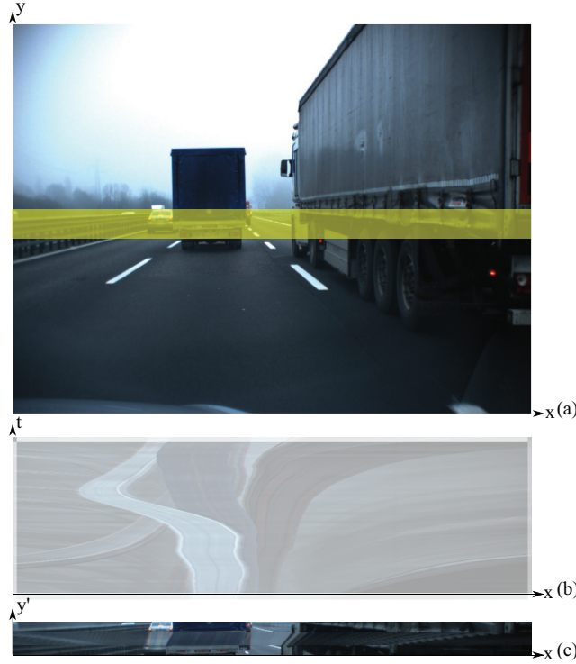
Figure 1. (a) The last frame from a 52 s long video sequence. The horizontal yellow belt is the vertical averaging region for the motion profile image. (b) Motion profile image generated out of a video sequence for visualization. (c) Merging video frames and motion profile patch image ( MPPI ) results in motion frame image ( MFI ) for real-time processing. The horizontal axis is the same as the video frame, while the vertical axis, y' , is a mixture of spatial and temporal axes.
