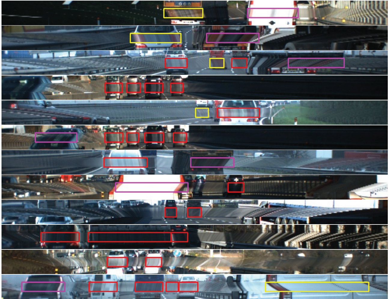
Figure 6. Vehicle labeling in the motion frame images. Bounding boxes are only drawn on the motion profile patch images. The color shows vehicle's motion directions; red: zero-flow, yellow: negative-flow, purple: positive-flow.
