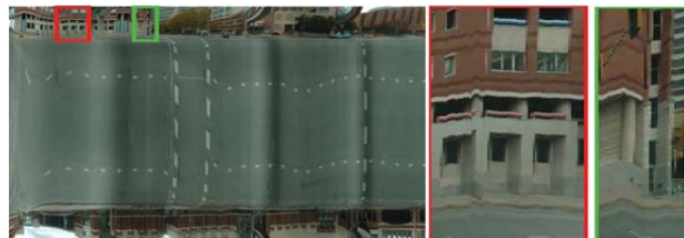
Figure 7. Camera yaw and roll cause shape deformation due to vehicle shaking. In enlarged partial views, lines are vertically zigzagged.
