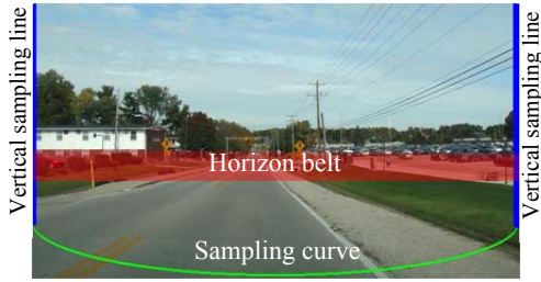
Figure 1. A camera view and the locations of sampling curve and vertical lines on side margins. The horizon belt is colored in red.
