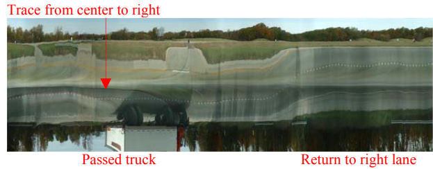
Fig 13. A passed vehicle's motion trajectory from center to right margin on the temporal profile.
