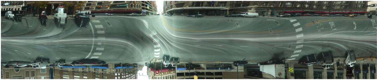
Figure 16. Urban driving in temporal profile. The caps and lane marks on the road surface are clearly recorded. The vehicle has a left turn from a one-way street to a two-way street, after changing from middle lane to left lane. The vehicle shifts to right lane after turning.
