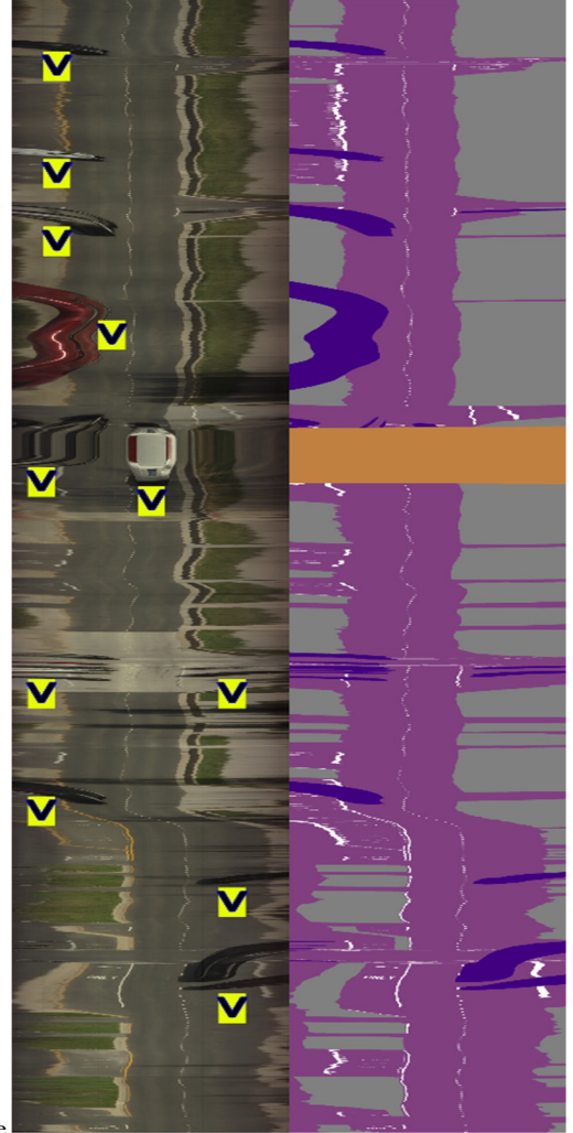
Road Profile Label Figure 4: Road profile and labels. The time axis is upward. The horizontal axes are the x axis in the image. Vehicle traces are marked with V signs. (a) Vehicle traces in motion and stopping are visible in the road profile. (b) We labeled six semantic classes from materials and motion styles for road profile.
