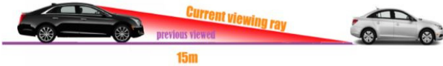
Figure 1: The plane of sight through the sampling line in the frame captures road information for driving. The space below the current rays is previously scanned. The degraded shading in red denotes the past observation space.
