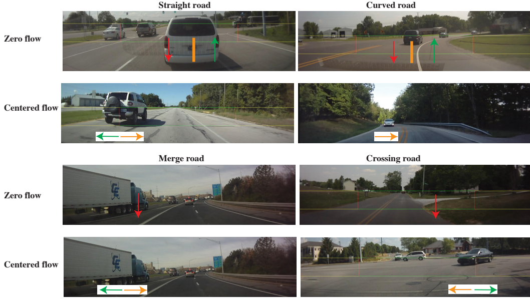
Fig. 3. Different road collision cases cause horizontal motion and vertical flow expansion. The red arrows indicate motion direction of potential collision, green arrows mean safe motion, and orange arrows mean centered motion direction requiring attention. The vehicle heading direction is at the image center.
