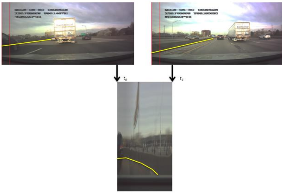
Figure 9 Example of scanning effect of lane change event in highway. Top images are first and last frames. Divergence of parallel lines to the heading direction is visible in the y profile in the bottom image. One curb line is highlighted in yellow both in frames and motion profile.
